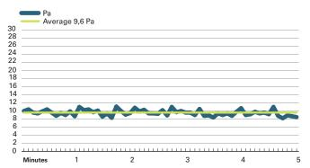
PRESSURE DROP SYSTEM (C-D) FILTER WITH DISTRIBUTOR PLATE 8 L/S
